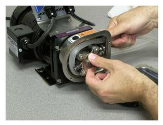
5. Align marks on tubing with inside edge of pump housing.
