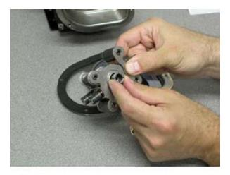
Clean inside of pump housing with damp rag or an appropriate cleaning solution to remove any chemical or tubing residue.
