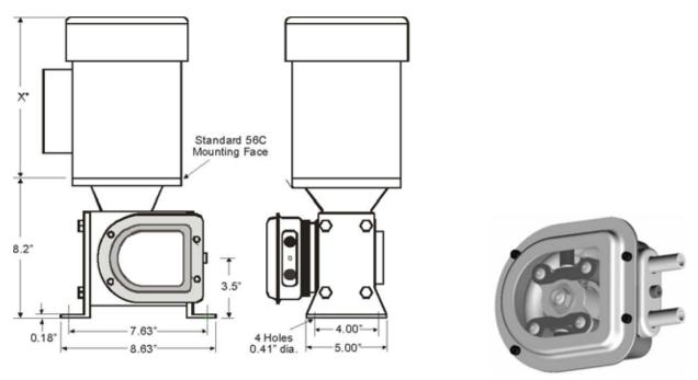
The PERIDOS Series pumphead has two spring-loaded working rollers, which automatically compensate for minor variations in tubing wall thickness, giving extended tube life.
