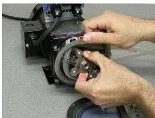
5. Remove worn pump tubing from pumphead.
