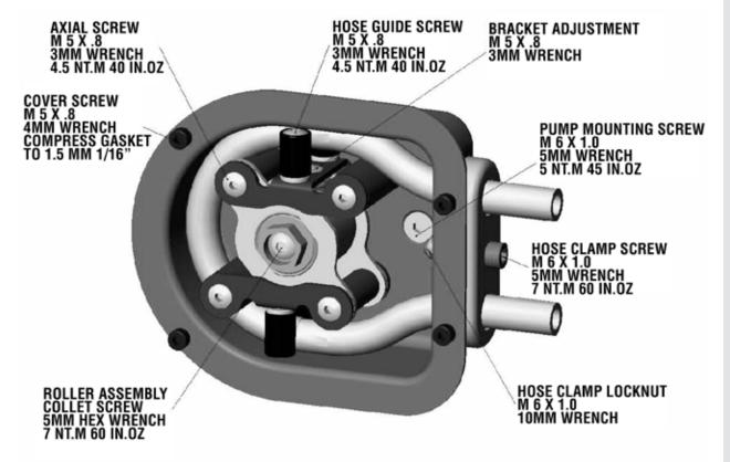
IMPORTANT: The PERIDOS Series is equipped with a pump cover for safety and protection against chemical spills. The cover must be installed whenever the pump is in use.
