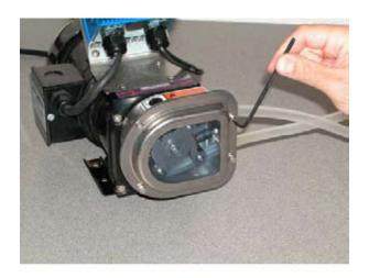
2. Loosen Tube Seal Clamp Screw with 5mm hex wrench.
