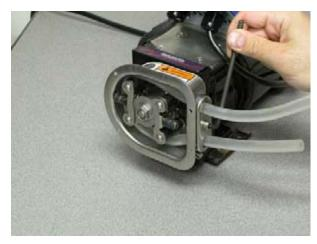
8. Inspect pump cover gasket. Replace if damaged. Reinstall pump cover gasket and cover. 11.5 inches
