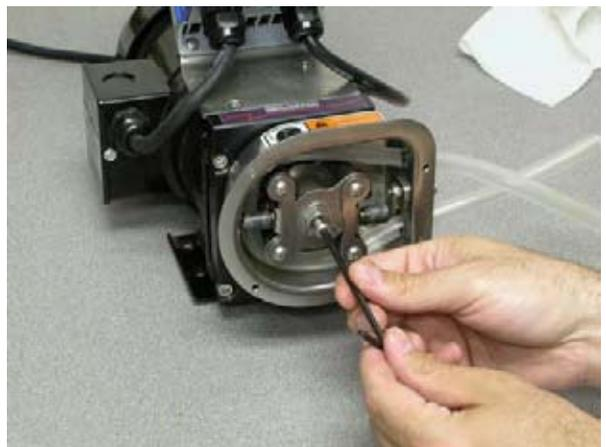
7. Tighten hose seal clamp screw. Be sure to tighten firmly to prevent "tubing walk." Tubing walk can occur when the hose seal is the wrong size or is not sufficiently tight to keep the rollers from pulling the hose through the pump as it rotates.
