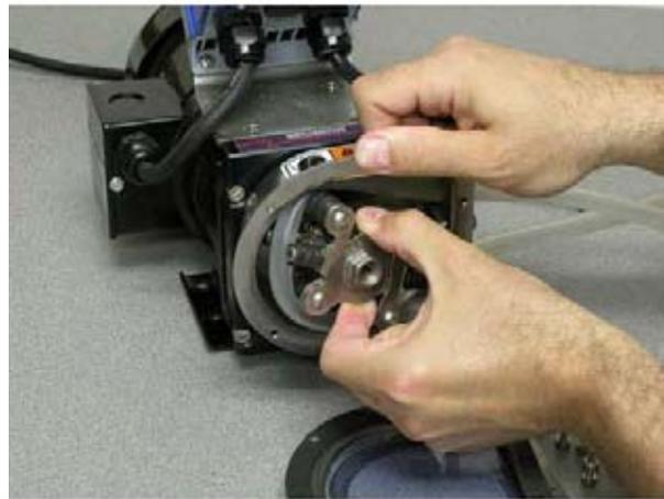
5. Remove worn pump tubing from pumphead.
