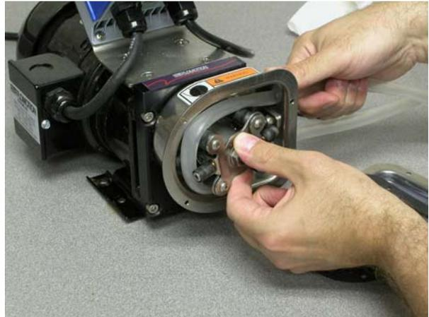
5. Align marks on tubing with inside edge of pump housing.
