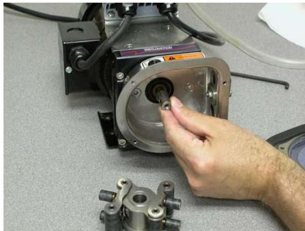
2. Mark an 11.5" section of hose, which will be the portion contained within the pump. Leave sufficient excess on the suction and discharge sides of the pump for the desired connections. If you leave the excess intake hose in a coil near the pump it will make it easy to feed a new section of hose through the rollers when the section in the pump becomes worn.
