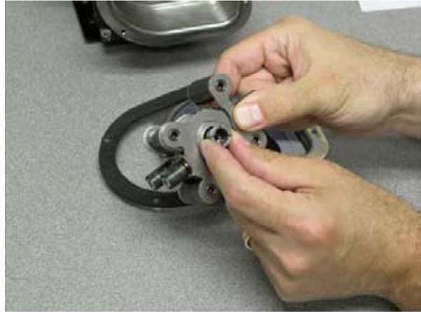
7. Clean inside of pump housing with damp rag or an appropriate cleaning solution to remove any chemical or tubing residue.
