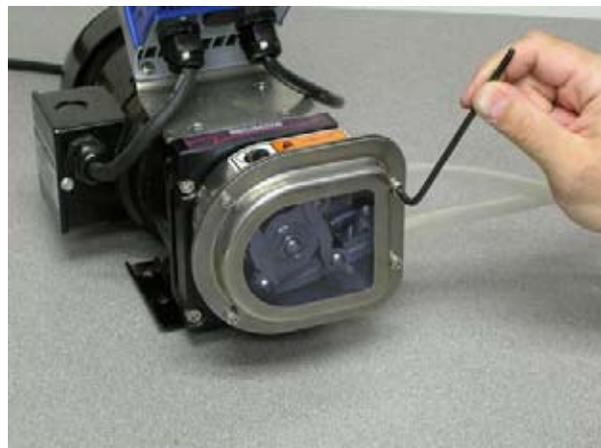
*11.5 inches of hose is the length required inside the pump housing.*
