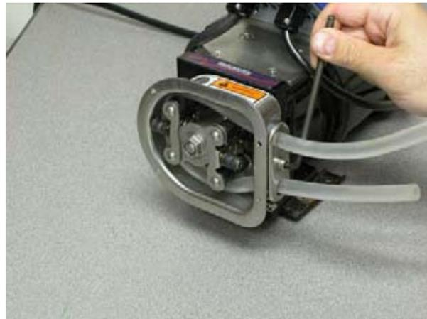
8. Inspect pump cover gasket. Replace if damaged. Reinstall pump cover gasket and cover. 11.5 inches
