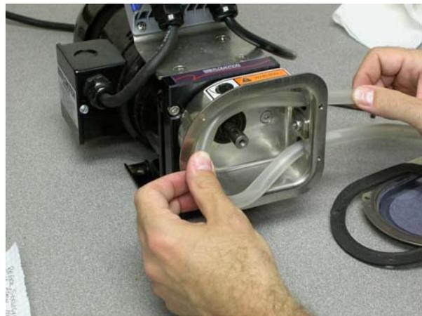
4. Loop tubing around roller assembly between guides as shown. Remove slack in tubing while rotating roller assembly and sliding onto collet.
