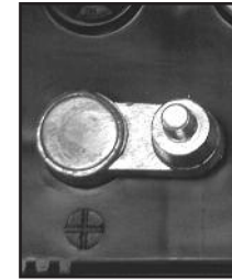
POSITIVE POST HAS LARGER DIAMETER
