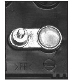
NEGATIVE POST HAS SMALLER DIAMETER
