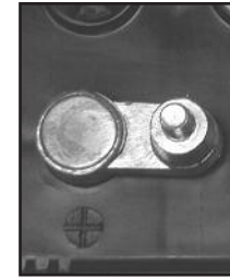
POSITIVE POST HAS LARGER DIAMETER
