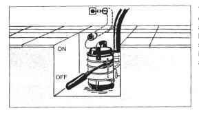
Your GF 32-9 comes equipped with a fully automatic on/off level switch as standard. The pump is easily installed in a sump.
