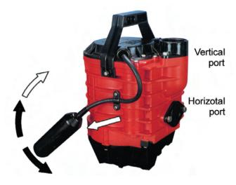
The unique dual port design virtually eliminates kinks in your hose; use vertical port for deep/narrow places or use the horizontal port for shallow/wide applications.
