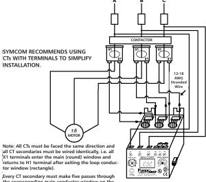
the corresponding main conductor window on the Model 777-KW/HP.
