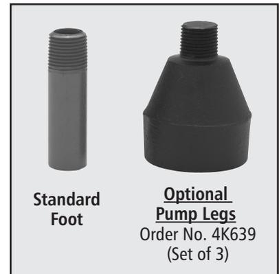
\* Optional pump legs are recommended for poly or fiberglass basin installations where the pumps contact the basin floor. The order number for a package of (3) three optional pump legs is 4K639.
