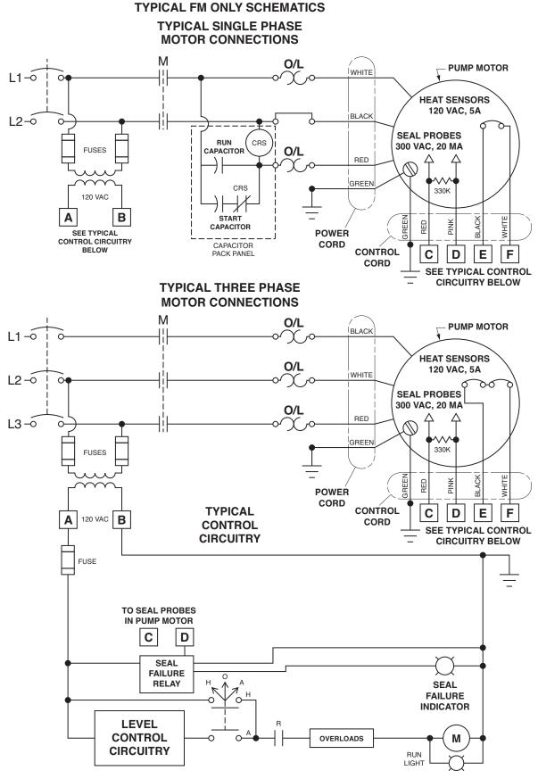
NOTE: CAPACITORS AND/OR CONTROLS SHOULD BE LOCATED OUTSIDE HAZARDOUS AREA AND ENCLOSED IN AN APPROPRIATE ENCLOSURE.
