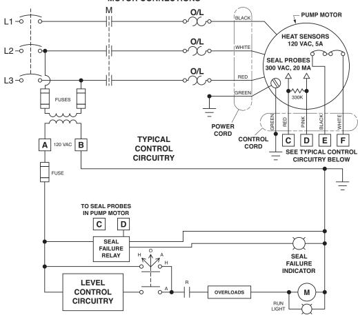
NOTE: CAPACITORS AND/OR CONTROLS SHOULD BE LOCATED OUTSIDE HAZARDOUS AREA AND ENCLOSED IN AN APPROPRIATE ENCLOSURE.
