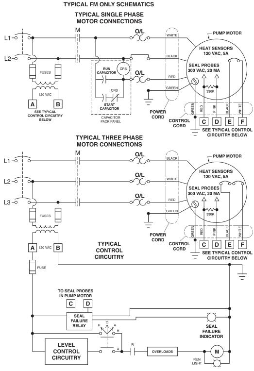
NOTE: CAPACITORS AND/OR CONTROLS SHOULD BE LOCATED OUTSIDE HAZARDOUS AREA AND ENCLOSED IN AN APPROPRIATE ENCLOSURE.
