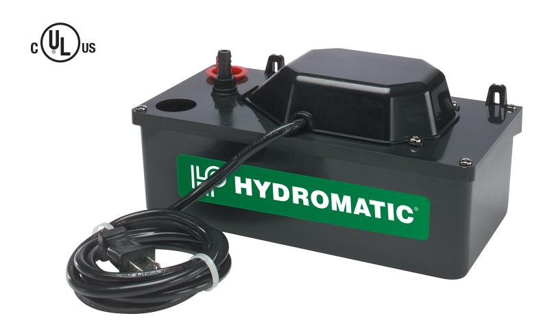
The Hydromatic Condensate units are designed to automatically remove the liquid from an air conditioner evaporative coil and/or a gas condensing warm air furnace. These units are made from a tough ABS plastic so they will resist corrosion and impacts.
