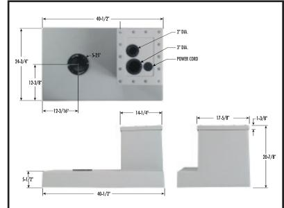
All dimensions in inches. Component dimensions may vary ± 1/8 inch. Dimensional data not for construction purpose unless certified. Dimensions and weights are approximate. On/Off level adjustable. We reserve the right to make revisions to our product and their specifications without notice.
