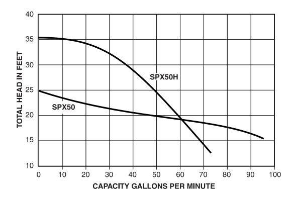
The curves reflect maximum performance characteristics without exceeding full load (Nameplate) horsepower. All pumps have a service factor of 1.2. Operation is recommended in the bounded area with operational point within the curve limit. Performance curves are based on actual tests with clear water at 70° F. and 1280 feet site elevation.
