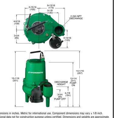
All dimensions in inches. Metric for international use. Component dimensions may vary ± 1/8 inch. Dimensional data not for construction purpose unless certified. Dimensions and weights are approximate. On/Off level adjustable. We reserve the right to make revisions to our product and their specifications without notice
