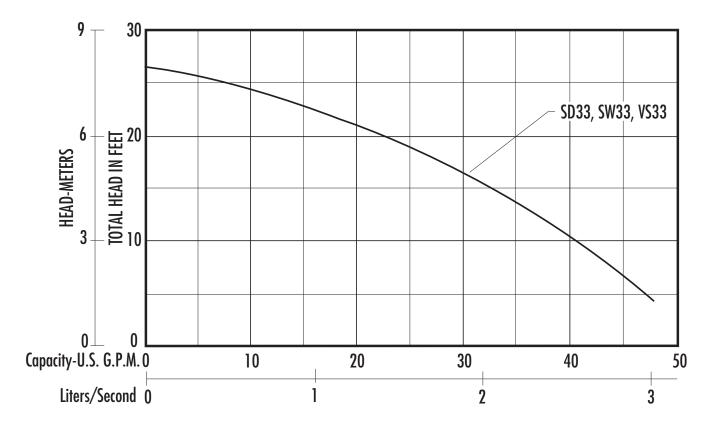
The curves reflect maximum performance characteristics without exceeding full load (Nameplate) horsepower. All pumps have a service factor of 1.2. Operation is recommended in the bounded area with operational point within the curve limit. Performance curves are based on actual tests with clear water at 70° F. and 1280 feet site elevation.
