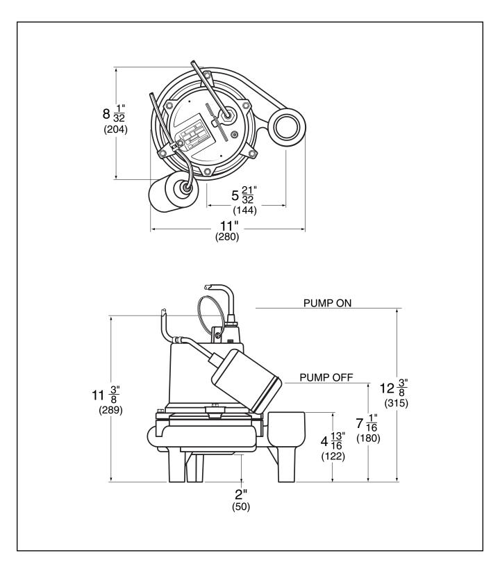
All dimensions in inches. Metric for international use. Component dimensions may vary  $\pm$  1/8 inch. Dimensional data not for construction purpose unless certified. Dimensions and weights are approximate. On/Off level adjustable. We reserve the right to make revisions to our product (s) and the product (s) specifications without notice.
