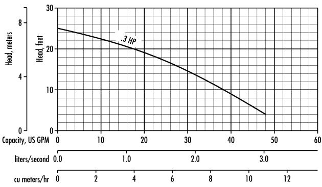
The curves reflect maximum performance characteristics without exceeding full load (Nameplate) horsepower. All pumps have a service factor of 1.2. Operation is recommended in the bounded area with operational point within the curve limit. Performance curves are based on actual tests with clear water at 70° F. and 1280 feet site elevation.
