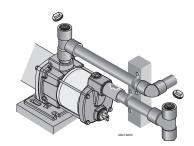
Figure 13 – Remove Priming Plug
