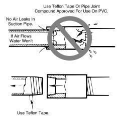
Figure 4 - Suction Pipe Must Not Leak
