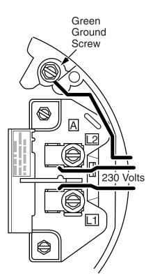
Figure 12A – 230V Single Phase Wiring Diagram
