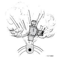
Figure 15 – Do Not Run Pump with Discharge Shut-off.
