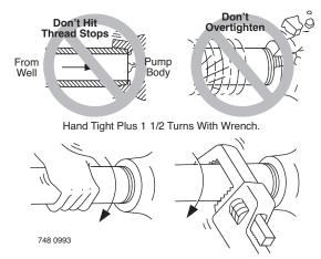
Figure 11 – Don't overtighten.
