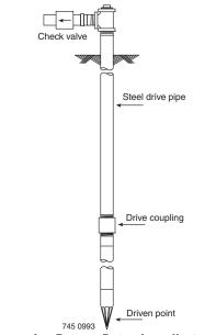
Figure 6 – Driven Point Installation
