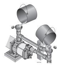
Figure 14 – Fill Pump Before Starting
