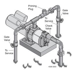
Figure 7 – Multiple Discharge
