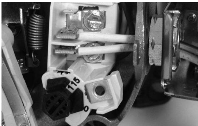
Figure 7: Voltage set to 115 volts, Dial Type
