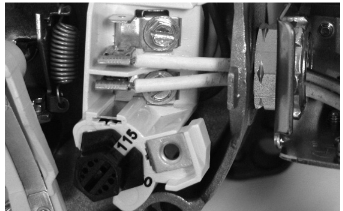
Figure 9: Voltage set to 115 volts, Dial Type
