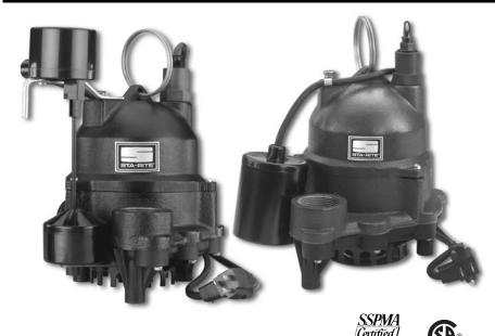
Rugged cast iron sump pumps feature a vortex impeller to provide solids-handling capability up to 1/2". Product is available in 1/3 or 1/2 HP, 115 Volt single phase 60 Hz. Pump discharge is 1-1/2" FNPT. Field-replaceable piggy-back float switch: vertical for minimum diameter 10" sumps, or tethered for minimum diameter 14" sumps.
