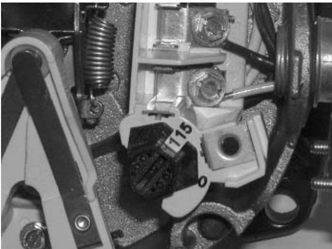
Figure 6: Motor Set for 115 Volt Operation.
