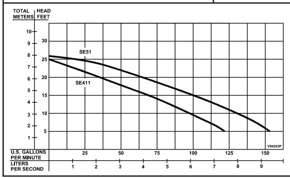
Testing is performed with water specific gravity of 1.0 @ 68°F (20°C), other fluids may vary performance
