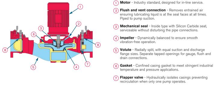
8 **Isolation valves** - Allow one unit to be isolated and removed for service while the second unit remains in operation.
