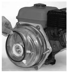
Figure 32: Remove front O-Ring
