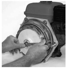
Figure 52: Fasten Impeller
