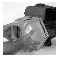
Figure 31: Remove Casing
