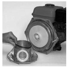
Figure 9: Remove casing O-Ring
