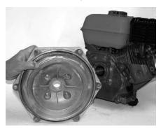
Figure 42: Remove Seal Plate and Seals
