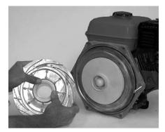
Figure 20: Install Impeller Wear Ring
