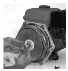
Figure 36: Remove Spacer
