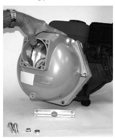
Figure 56: Install Support Foot
