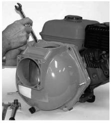
Figure 5:Casing Nut Removal
