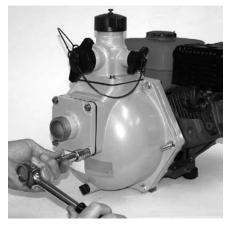
Figure 59: Tighten Suction Housing
