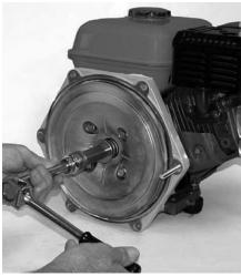
Figure 40: Remove Shaft Extension
