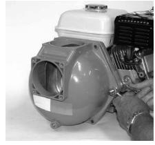
Figure 23: Fasten Casing
