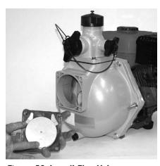
Figure 58: Install Flap Valve
