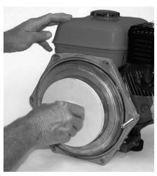
Figure 19: Install Impeller
