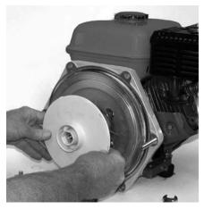
Figure 38: Remove Second Impeller
