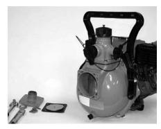
Figure 2: Suction Flange Removal
