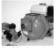
Figure 25: Fasten Suction and Discharge Flanges
