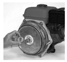
Figure 51: Insert Diffuser O-Ring
