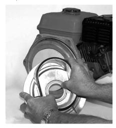
Figure 8: Remove Impeller Wear Ring
