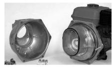
Figure 6: Remove Casing
