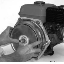
Figure 37: Remove Second Diffuser
