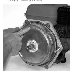
Figure 50: Locate Diffuser
