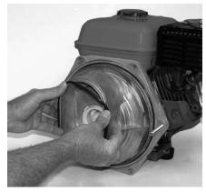
Figure 21: Install Diffuser
