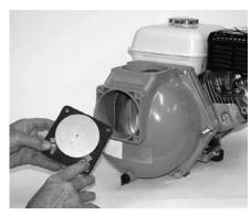
Figure 24: Install Flap Valve
