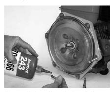
Figure 46: Install Seal plate Bolts
