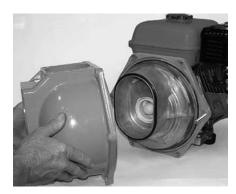
Figure 22: Fit Casing
