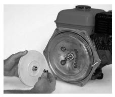
Figure 18: Install Rotating Seal
