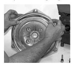
Figure 44: Prepare Seal Plate
