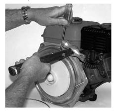
Figure 10: Remove Impeller
