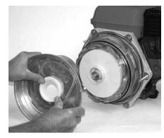
Figure 53: Install Wear Ring
