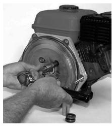
Figure 41: Remove Seal Plate Bolts
