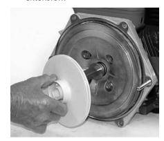
Figure 48: Install First Impeller
