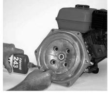
Figure 16: Fasten Seal Plate to Engine
