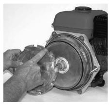
Figure 52: Install Front Diffuser
