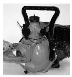
Figure 1: Suction Flange Removal
