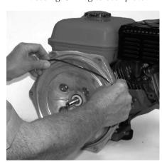
Figure 17: Install casing O-Ring
