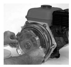
Figure 35: Remove Front Diffuser
