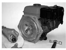
Figure 11: Remove Rotating Seal
