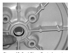
Figure 45: Seal Plate Drain Location
