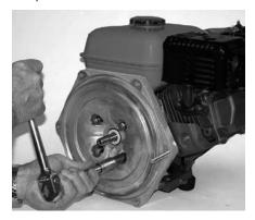
Figure 12: Seal plate Removal
