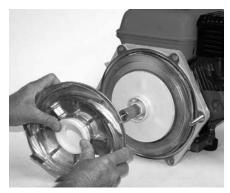
Figure 49: Install Diffuser
