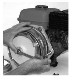
Figure 34: Remove Impeller
