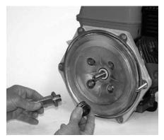
Figure 47: Install Seal and Extension
