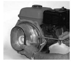
Figure 7: Remove Diffuser
