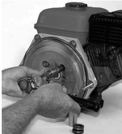
**Figure 41: Remove Seal Plate Bolts**
