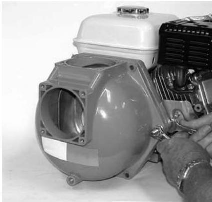
**Figure 23: Fasten Casing**
