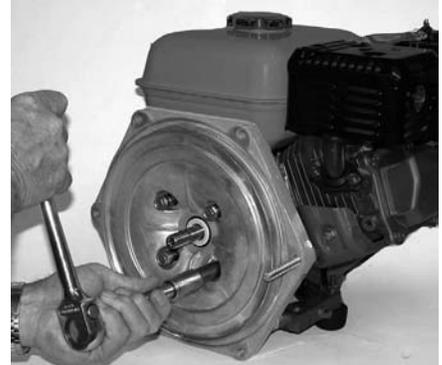
**Figure 12: Seal plate Removal**
