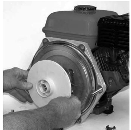
**Figure 38: Remove Second Impeller**
