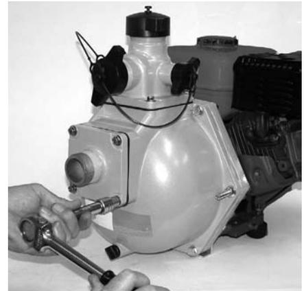
**Figure 59: Tighten Suction Housing**
