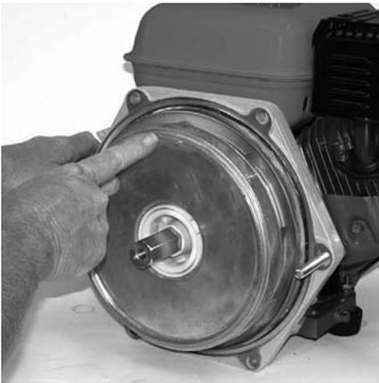
**Figure 50: Locate Diffuser**
