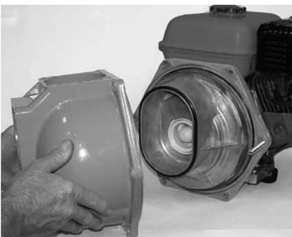
**Figure 22: Fit Casing**
