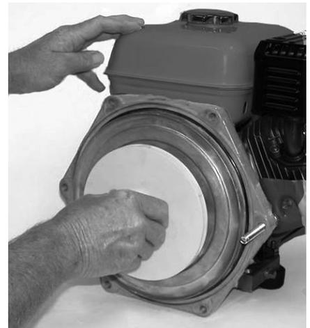
**Figure 19: Install Impeller**
