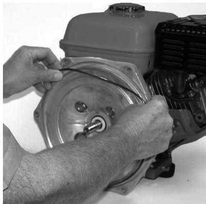
**Figure 17: Install casing O-Ring**
