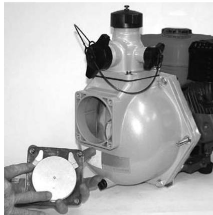
**Figure 58: Install Flap Valve**
