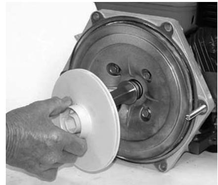
**Figure 48: Install First Impeller**
