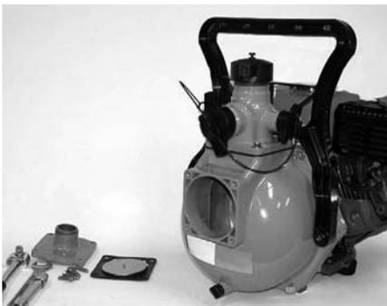
**Figure 2: Suction Flange Removal**
