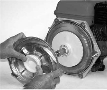
**Figure 49: Install Diffuser**
