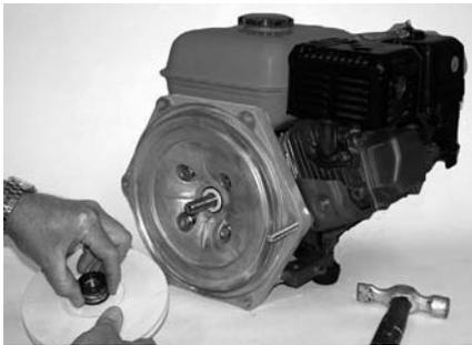
**Figure 11: Remove Rotating Seal**
