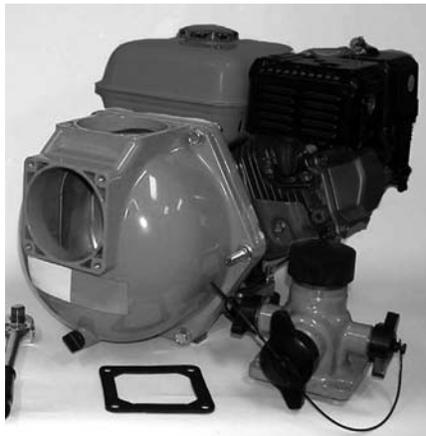
**Figure 4: Remove discharge Assembly**
