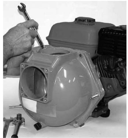
**Figure 5: Casing Nut Removal**
