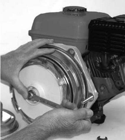
**Figure 34: Remove Impeller**
