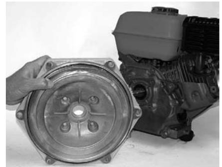
**Figure 42: Remove Seal Plate and Seals**
