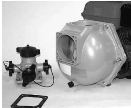
**Figure 57: Install Discharge Flange**
