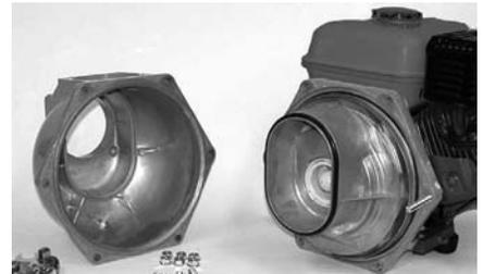
**Figure 6: Remove Casing**
