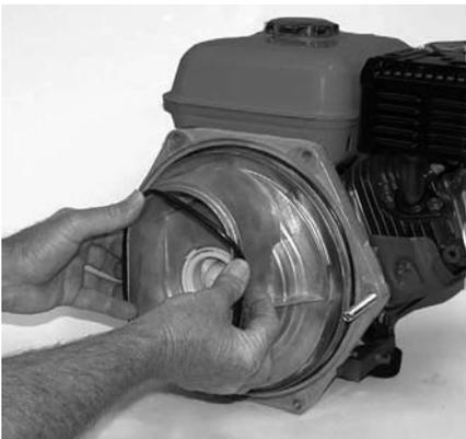
**Figure 21: Install Diffuser**
