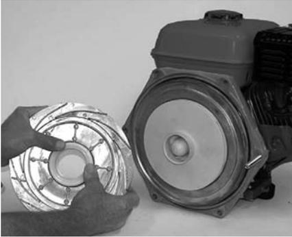
**Figure 20: Install Impeller Wear Ring**
