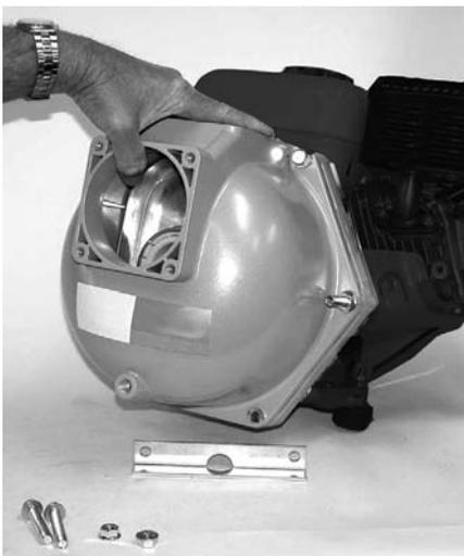
**Figure 56: Install Support Foot**
