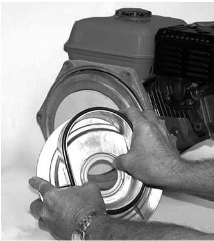
**Figure 8: Remove Impeller Wear Ring**
