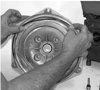
**Figure 44: Prepare Seal Plate**
