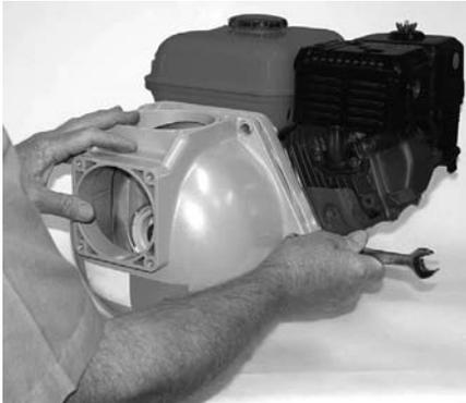
**Figure 55: Install Casing**
