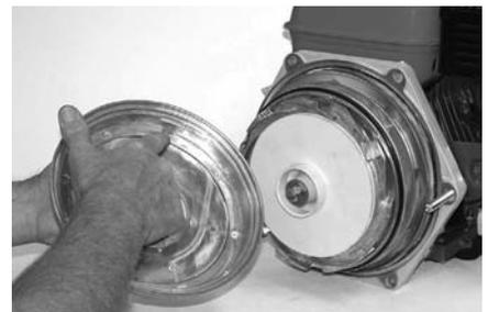
**Figure 54: Position Front Diffuser**
