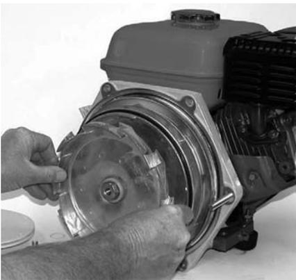
**Figure 35: Remove Front Diffuser**
