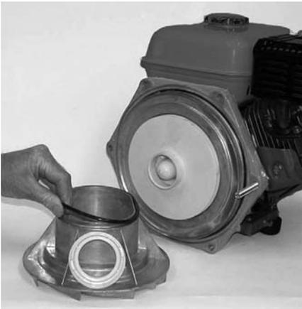
**Figure 9: Remove casing O-Ring**
