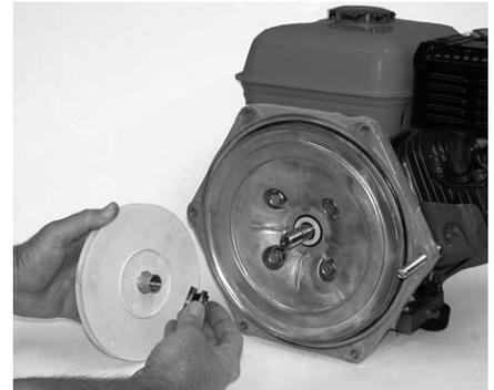
**Figure 18: Install Rotating Seal**
