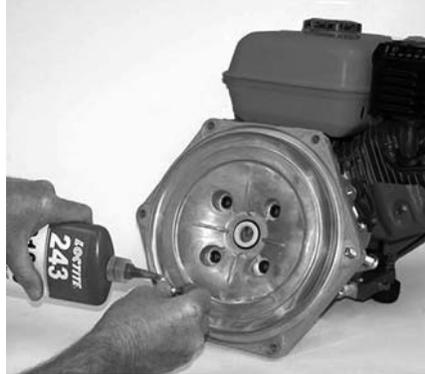
**Figure 16: Fasten Seal Plate to Engine**
