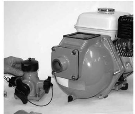
**Figure 25: Fasten Suction and Discharge Flanges**
