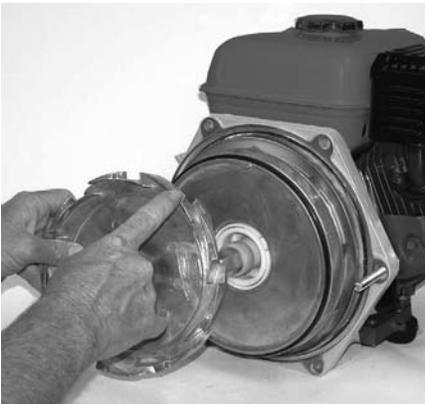
**Figure 52: Install Front Diffuser**
