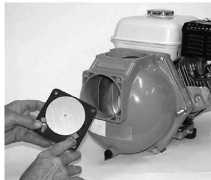
**Figure 24: Install Flap Valve**
