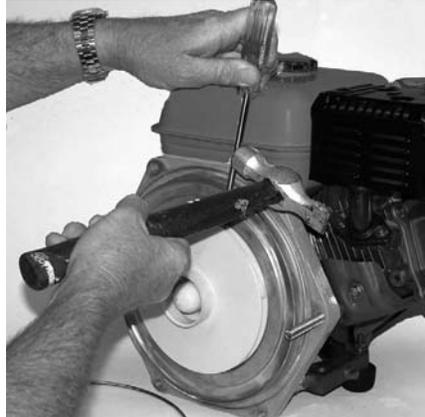
**Figure 10: Remove Impeller**
