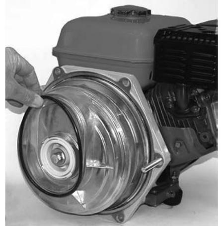
**Figure 32: Remove front O-Ring**
