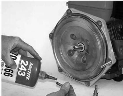
**Figure 46: Install Seal plate Bolts**
