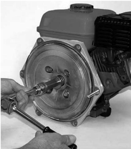
**Figure 40: Remove Shaft Extension**
