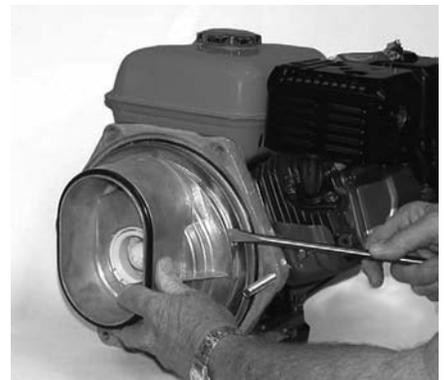
**Figure 7: Remove Diffuser**
