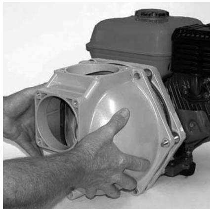
**Figure 31: Remove Casing**
