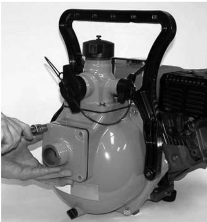
**Figure 1: Suction Flange Removal**
