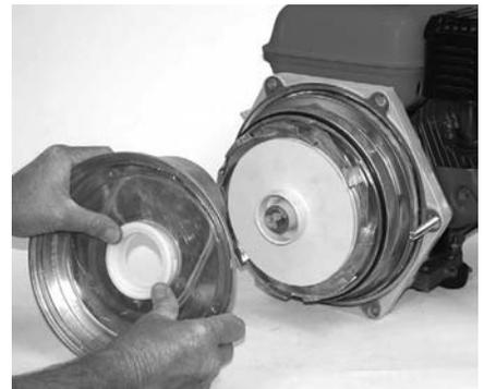
**Figure 53: Install Wear Ring**
