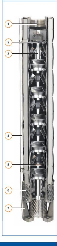
BERKELEY 6TS SERIES PUMPS feature heavy-duty 304 stainless steel construction and hard chrome wear surfaces that will outperform ordinary fabricated stainless steel pumps in aggressive water conditions. The stateof-the-art design includes 100% lead-free components with high efficiency performance in 6 hydraulics up to 400 GPM and 60 HP.
