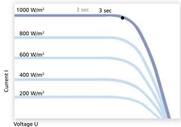
Typical Current-Voltage-curve of a photovoltaic panel. By employing MPP tracking every three seconds, the Ecocirc DC pumps always automatically achieve maximum performance at any given insolation.
