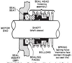
FIGURE 3a: End Face Mechanical Seal
