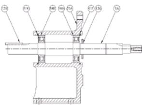
Figure 4A Bearing Frame Assembly
