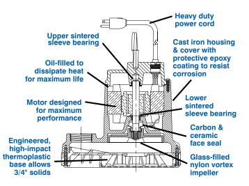
The Model 8E-CIA-VDS De-watering and Effluent pumps are for residential and light commercial use. Pumps feature a 1-1/2" FNPT discharge with a maximum head of 21' and ABS base.
