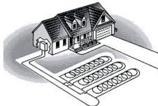
Figure 3: Horizontal piping layout for Ground Source Heat Pump installation. [ref: Jackson Electrical Membership Corporation]
