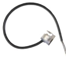
**AQS-1/2 (Part No. 113223) and AQS-3/4 (Part No. 113224) Aquastat—** are designed to thermostatically turn any B&G NBF circulator ON and OFF. The AQ-1/2 or AQ-3/4 will switch the pump OFF at 120°F (48.9°C) and ON at 100°F (37.8°C). The aquastats are available in separate models that will sense the temperature for either 1/2" or 3/4" copper pipe.
