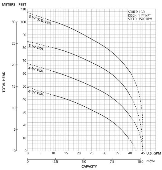
= A 1<sup>1</sup>/<sub>4</sub>" minimum discharge pipe requires a minimum flow of 10 gpm to maintain a 2 ft./sec. scouring velocity. Flows less than 10 gpm will allow solids to settle in the pipe.
