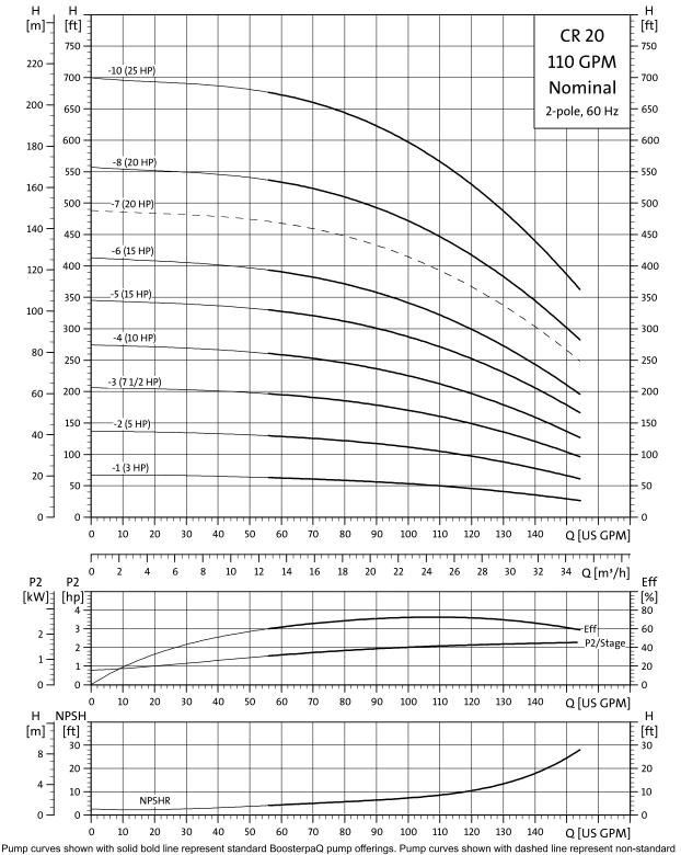
Pump curves shown with solid bold line represent standard BoosterpaQ pump offerings. Pump curves shown with dashed line represent non-standa BoosterpaQ pump offerings, which are available upon request.
