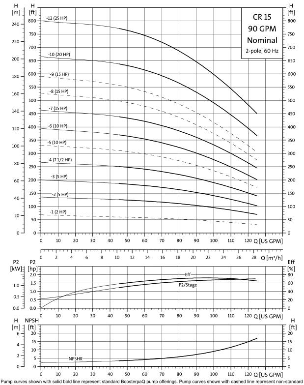
Pump curves shown with solid bold line represent standard BoosterpaQ pump offerings. Pump curves shown with dashed line represent no BoosterpaQ pump offerings, which are available upon request.
