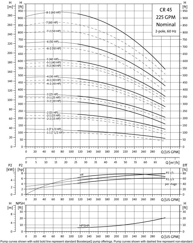
Pump curves shown with solid bold line represent standard BoosterpaQ pump offerings. Pump curves shown with dashed line represent non-standard BoosterpaQ pump offerings, which are available upon request.
