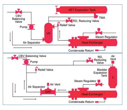
expansion and contraction caused by temperature variations. Units can be connected to any steam boiler or system, however, the capacity of the boiler must be sufficient to handle the load imposed by the heat exchanger. In addition, some method of controlling the flow to the exchanger must be provided and installed according to the manufacturer's directions.
