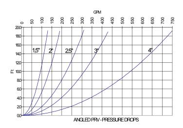
Figure 5. PRV PRESSURE DROP CHART
